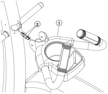
B. Using a 4mm allen wrench, attach the bullhorn to the console mast using 5 screws.
