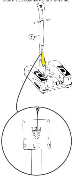
C. Using a 6mm allen wrench and a 17mm box end wrench, attach the console mast to the base using 6 hex screws and 3 lock nuts.
