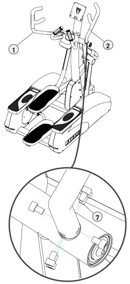
B. Using a Phillips screwdriver, attach the upper pivot covers to the swing arm assembly using 10 screws.
