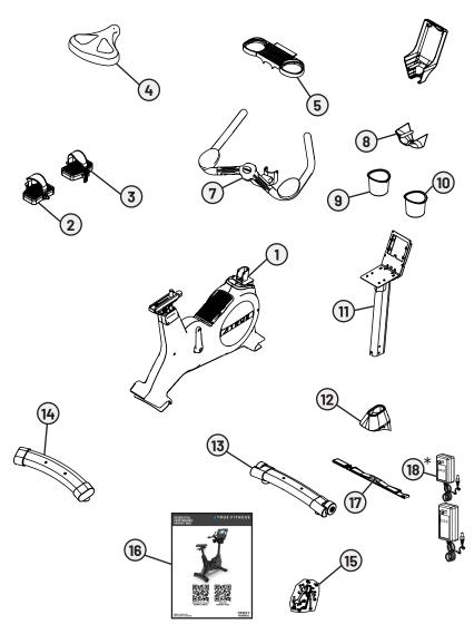
\*The 9V, 1.3A power adapter is for LED consoles only. Touchscreen consoles require a 12V, 3A power adapter, which is included with touchscreen consoles.
