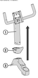
C. Pull the cables coming from the front of the bike through the front mast using the provided pull tie.
