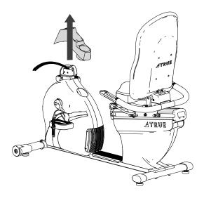
B. Slide the bottom console cover and bottle holder up the console mast.
