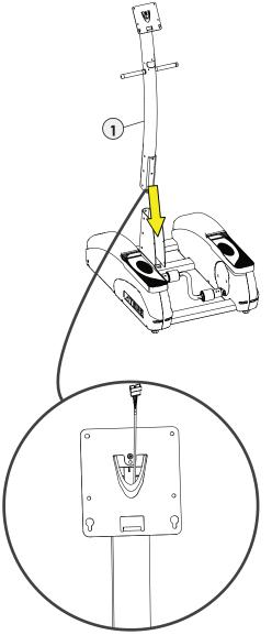
C. Using a 6mm allen wrench and a 17mm box end wrench, attach the console mast to the base using 6 hex screws and 3 lock nuts.
