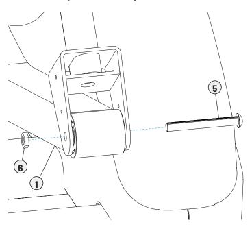
**NOTE:** Ensure that the pedal tubes are aligned on the center of the crankshaft rollers before tightening.
