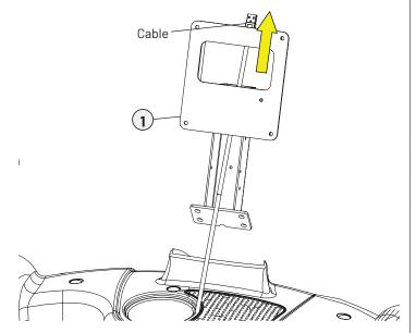
B. Using a 6mm ball end allen wrench, attach the console mast using 4 hex screws.
