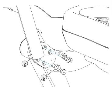
B. Using a #2 Phillips screwdriver, attach the exercise arm covers using 4 screws.
