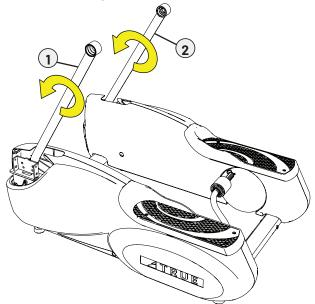
C. Using a 8mm allen wrench, insert 2 hex screws through the shroud and into the joint and tighten. Place 2 rubber caps over the holes in the shrouds.
