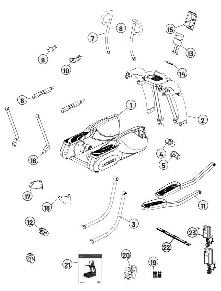
\*The 9V, 1.3A power adapter is for LED consoles only. Touchscreen consoles require a 12V, 3A power adapter, which is included with touchscreen consoles.
