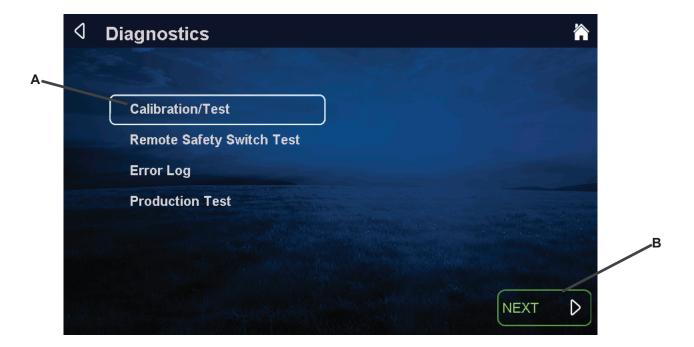
4. Under Calibration/Test, select **Speed/Incline Cal** (A) to highlight it. Press **NEXT** (B) to continue.
