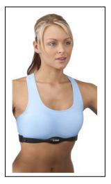
Initially the transmission signal for heart rate may be erratic or non-existent. Some moisture is necessary between the strap and the user's skin for proper transmission. Sweat from exercise works best, but ordinary tap water may be used prior to the workout if desired.
