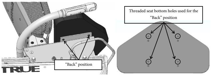
The default seat bottom position is towards the back, creating a minimal amount of space between the seat bottom and the mesh seat back.
