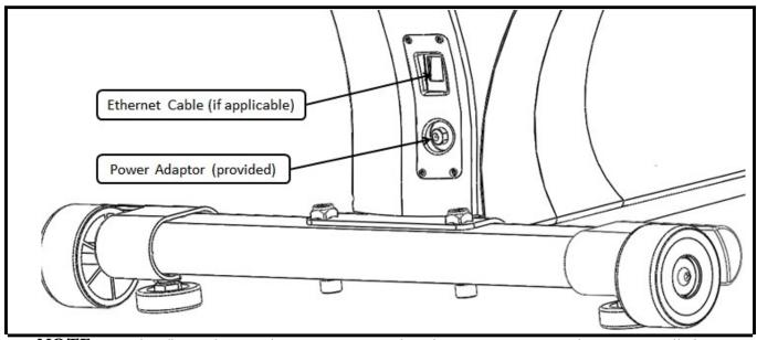
**NOTE:** For the 9" Touch Console, it is important that the 12V, 3A Power Adaptor is installed
