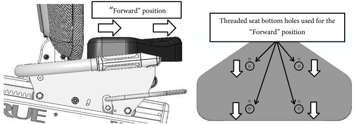
To adjust the seat bottom position forward, creating more room between the seat bottom and the mesh seat back, complete the following steps:
